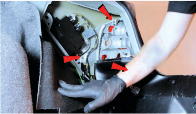
7) Remove [3x] 8mm nuts securing the tail light to the body.
