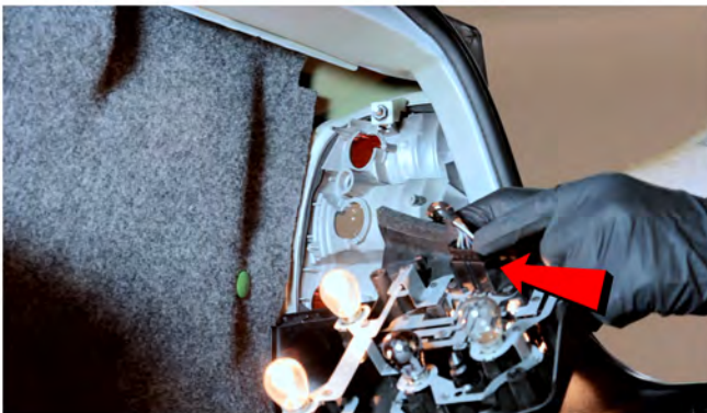
3) Disconnect the tail light wiring harness.
