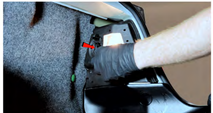
2) Unscrew the thumbscrew securing the bulb panel.
