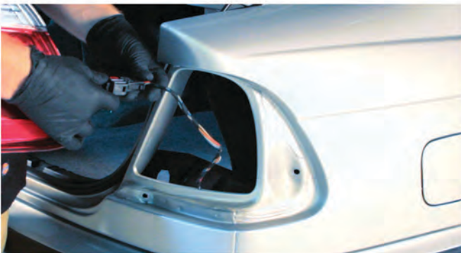
9) Locate your Spyder outer tail light. Connect the Spyder outer tail light to the tail light wiring harness.
