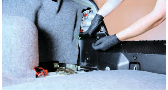
6) Pop out the round plastic plug covering an 8mm nut.
