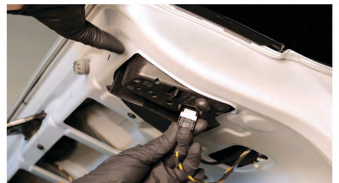
22) Reconnect the inner tail light wiring harness to the bulb plate.
