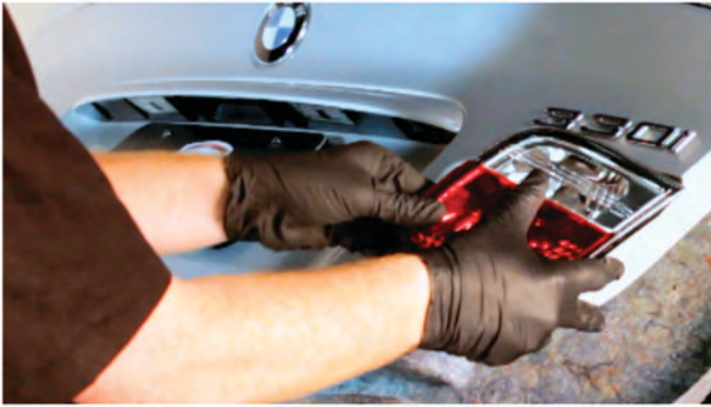
19) Seat the Spyder inner tail light. Carefully snap its retainer hook over the edge of the decklid.
