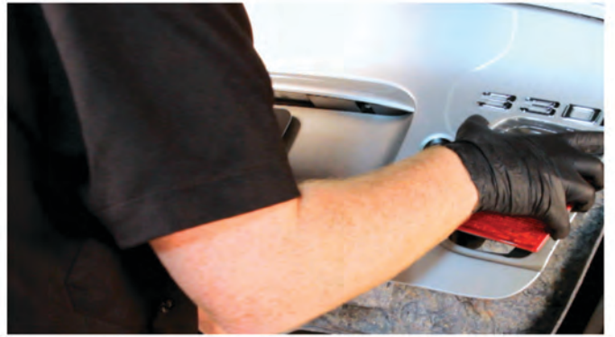
18) Unseat the OEM inner tail light by carefully easing its retainer hook off the edge of the decklid.
