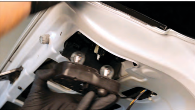
21) Reinstall the inner tail light bulb plate.
