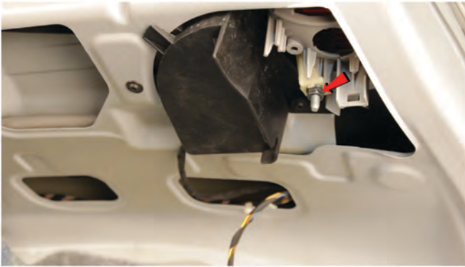
17) Remove [1x] 10mm nut and spacer securing the inner tail light.
