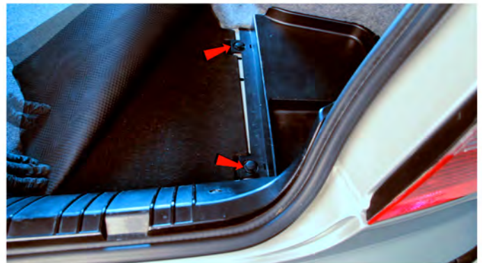
4) Peel back the trunkliner carpet and remove the two plastic retainers securing the battery cover panel.
