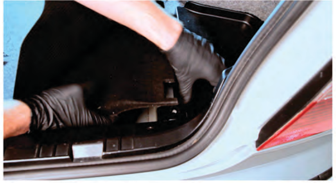
12) Reinstall the battery cover panel and secure it with [2x] plastic retainers, then replace the trunk liner.
