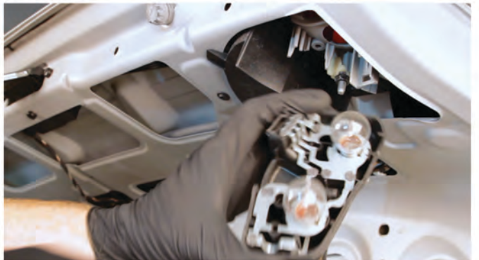
16) Squeeze the tab to release and remove the bulb panel.
