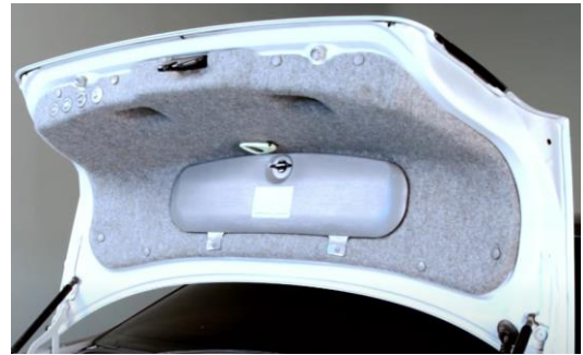
20. Reinstall tool kit thumb screw and (2x) Phillips screws to secure tool kit.
