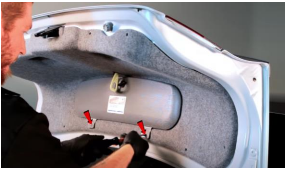
11. Remove (2x) phillips screws and thumb screw securing the tool kit.
