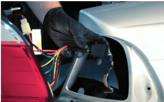
7. Connect Spyder outer tail light and seat light.
