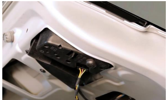
18. Next reinstall bulb plate to Spyder tail light and plug harness in.
