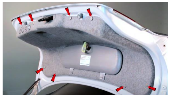
10. Moving on to inner tail light, remove (8x) retainers securing decklid liner with panel popper.
