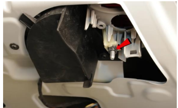
14. Remove (1x) 10mm nut securing inner tail light.
