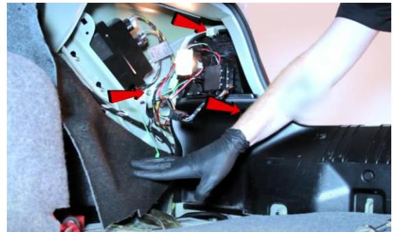
8. Reinstall (3x) 10mm nuts to secure tail light.
