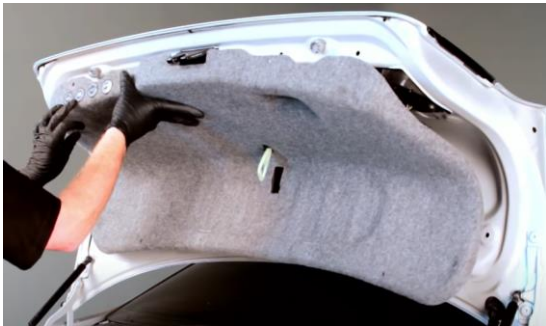
19. Reinstall deck lid and (8x) retainers to re-mount decklid.
