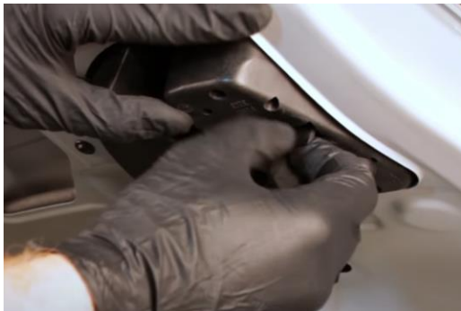
13. Push tab to release inner tail light bulb plate.
