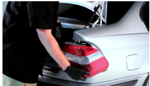
6. Unseat and remove outer tail light.
