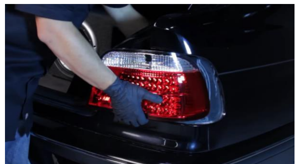
10. Seat Spyder tail light without harness to avoid pinching wiring.
