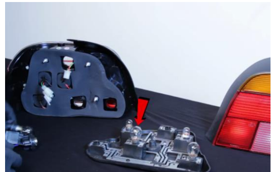
8. Remove reverse bulb from the bulb plate. Transfer bulb to Wht/Blk wire socket on Spyder harness.
