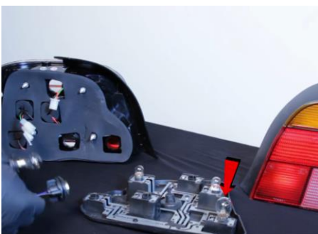
9. Remove rear fog lamp bulb from bulb plate. Transfer bulb to blue/blk wire socket on Spyder harness.
