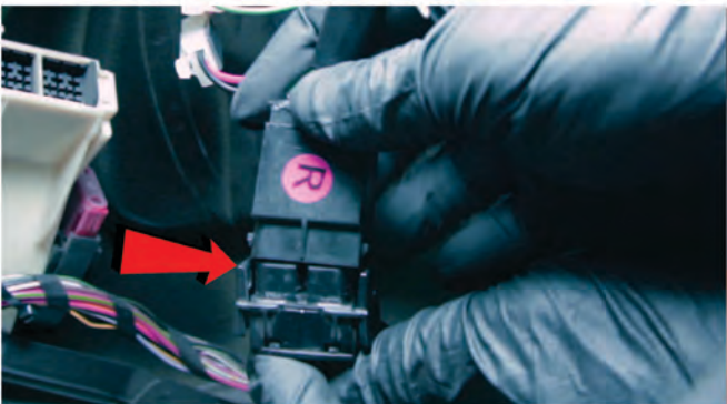
15) Reconnect the white wiring harness clips, red and black to red and black, green and black to green and black. Then reconnect the wiring harness.
