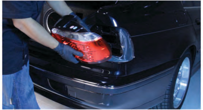
12) Seat the Spyder tail light. Seat the tail light without the harness connected to avoid pinching the harness between the tail light and body.
