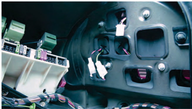
13) Reinstall [4x] 8mm nuts to secure the tail light to the body.
