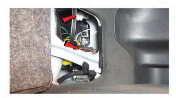
9) Reinstall the two plastic thumbscrews (white on top, black on the bottom), then close the access panel.
