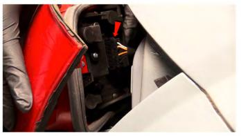
4) Disconnect the tail light wiring harness.
