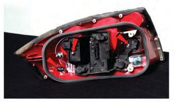
5) Remove [2x] Phillips screws securing the bulb plate to the tail light. Remove the side marker socket from the OEM tail light.
