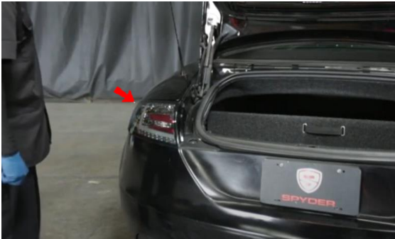
7. Push firmly on upper outside of tail light to snap in tail light.
