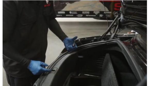
8. Reinstall retaining screw using multi tool.
