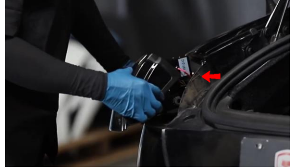
6. Make sure inner side of tail light slides over body panel.
