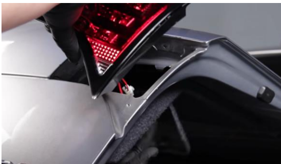
15. Seat inner tail light taking caution not to pinch harness between tail light and body.
