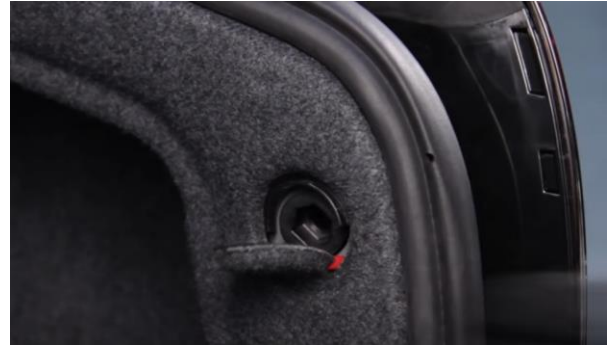
14. Seat outer tail light. Next, reinstall screw and replace round cover plug.
