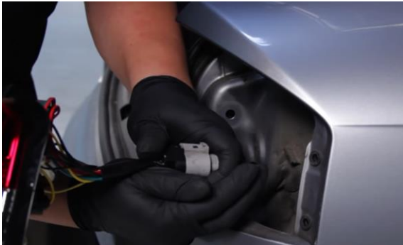
13. Connect wire harness to Spyder outer tail light.
