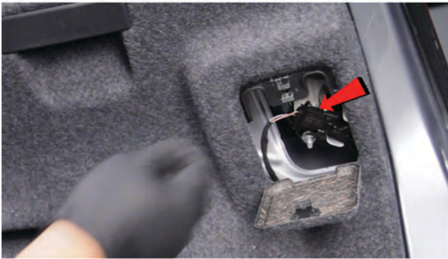
7) Disconnect the inner tail light harness.
