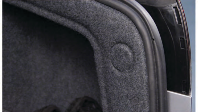
18) Reinstall the outer tail light screw cover.
