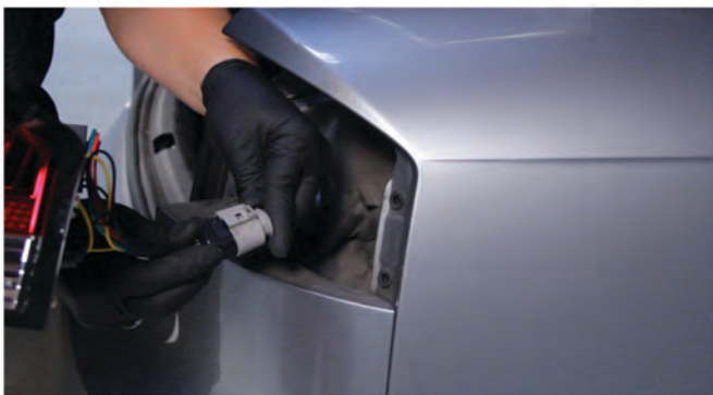
15) Connect the Spyder outer tail light to the wiring harness.
