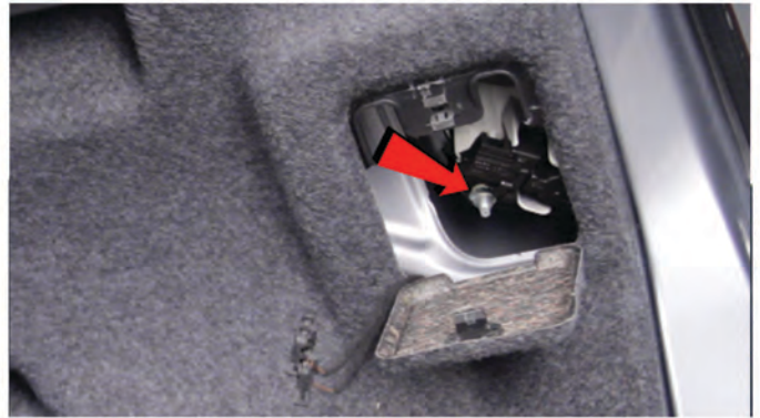
8) Remove [1x] 10mm nut and spacer securing the inner tail light.
