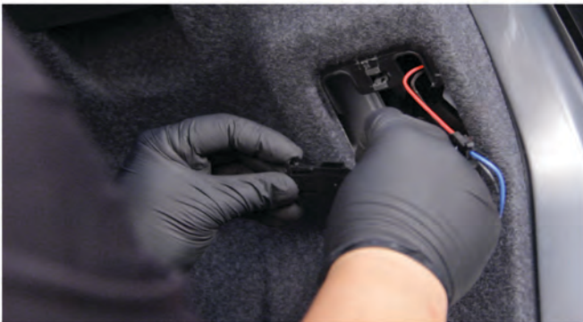
21) Connect the inner tail light wiring harness, then close the access cover.
