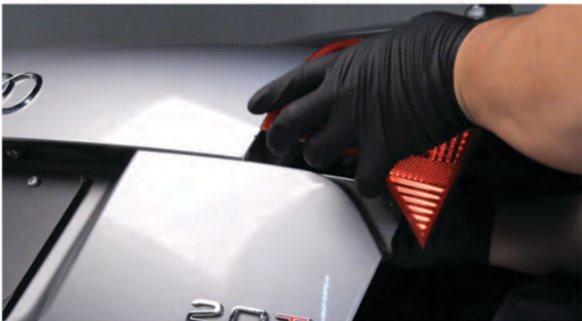
9) Unseat and remove the inner tail light.
