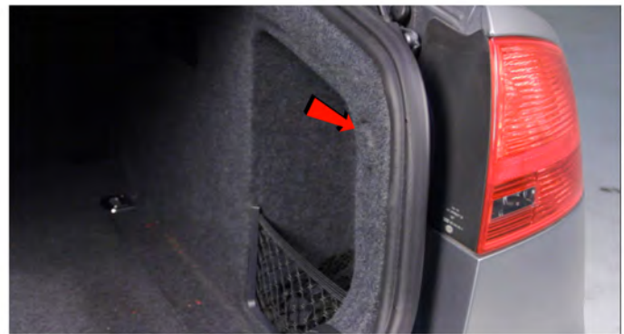
2) Remove the round cover plug in the trunk sill.
