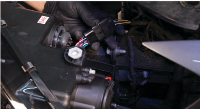
15) Connect the Spyder headlight to the headlight wiring harness.
