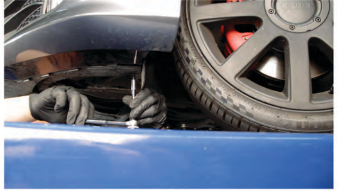
24) Reinstall [1x] T-15 torx screw securing the bottom corner of the fascia on each side.
