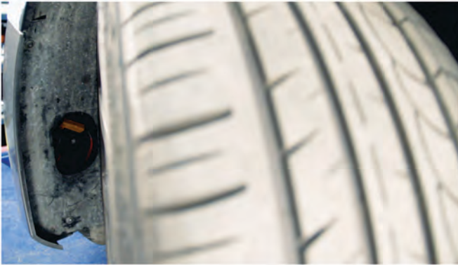
25) Reinstall [5x] T-15 torx screws to secure the fascia to the fender liner in the wheel well.
