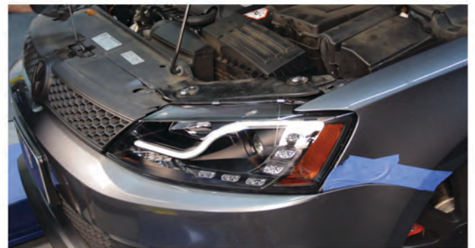
22) Reinstall [4x] T-15 torx screws to secure the grille.
