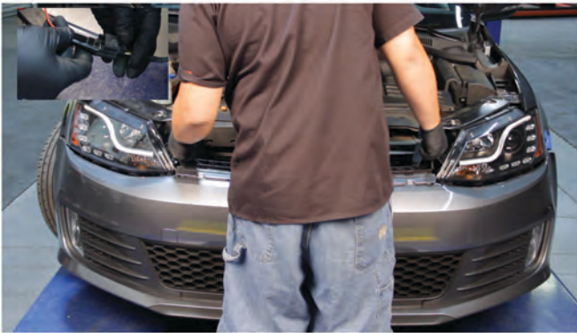
19) Reconnect the fog light harnesses [if equipped], then seat the front bumper fascia into its retaining hooks, then be sure the fascia edges clip properly into place.
