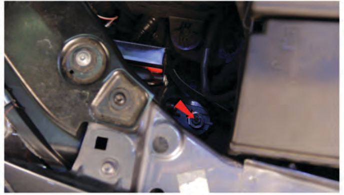
18) Reinstall [1x] T-30 Torx screw hidden behind the core support to secure the headlight.
