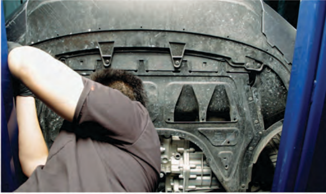
23) Reinstall [6x] T-15 torx screws to secure the fascia to the undertray.
