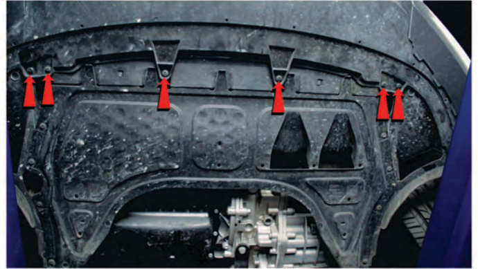
6) Remove [6x] T-15 torx screws securing the fascia to the undertray.
