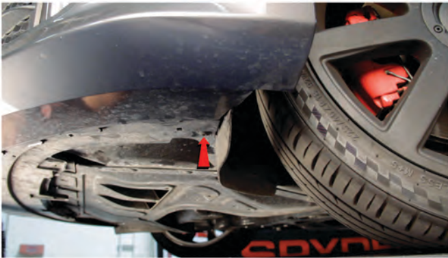
7) Remove [1x] T-15 torx screw securing the bottom corner of the fascia on each side.
