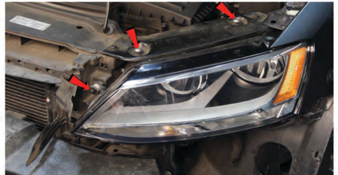
10) Remove [3x] T-30 torx screws securing the headlight.
