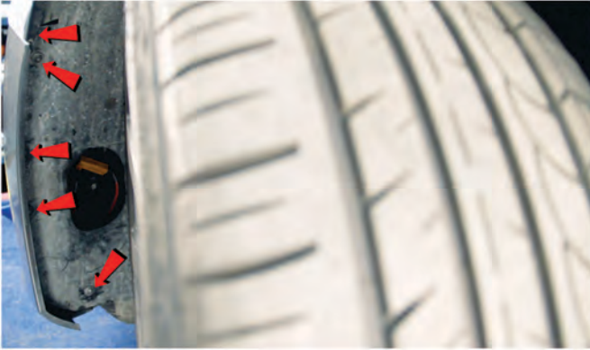
5) Remove [5x] T-15 torx screws securing the fender liner.
