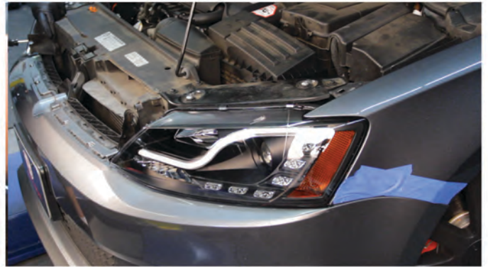
20) Reinstall [3x] T-30 torx screws hidden behind the grille to secure the fascia.
