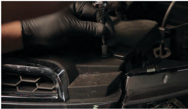
19) Reinstall [2x] 10mm bolts securing the fascia on either side of the grille.
