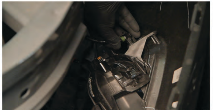
16) Reconnect the foglamp and sidemarker harnesses.
