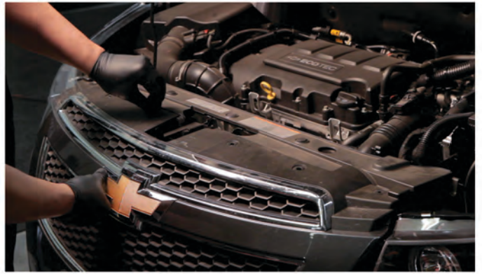
18) Reinstall [4x] plastic retainers to secure the front bumper fascia.
