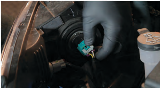
9) Disconnect the headlight wiring harness.
