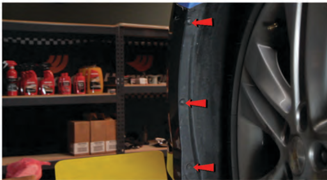
21) Reinstall [3x] T-15 torx screws securing the fender liner to the fascia.
