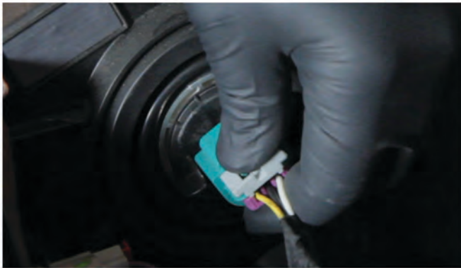
13) Reconnect the headlight wiring harness.
