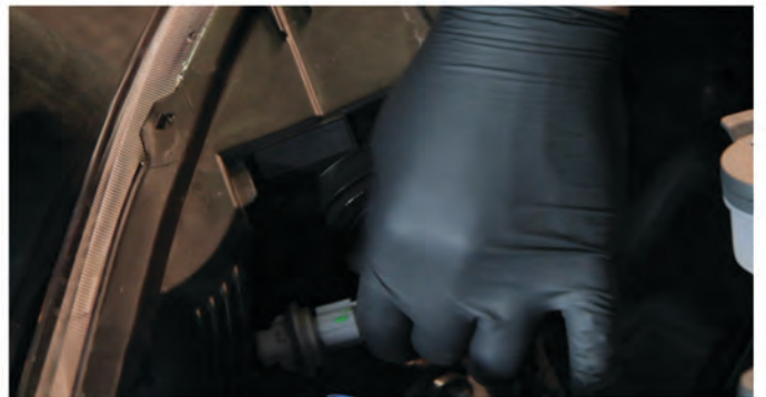
10) Disconnect the turn signal harness.
