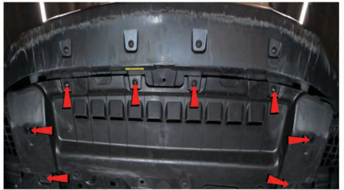
20) Reinstall [8x] T-15 torx screws to secure the fascia to the undertray.
