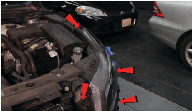
7) Remove [4x] 10mm bolts securing the headlight.
