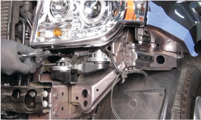
23) Reinstall [2x] 10mm bolts below the headlight to mount it.
