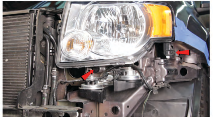
8) Remove [2x] 10mm bolts securing the headlight from below.
