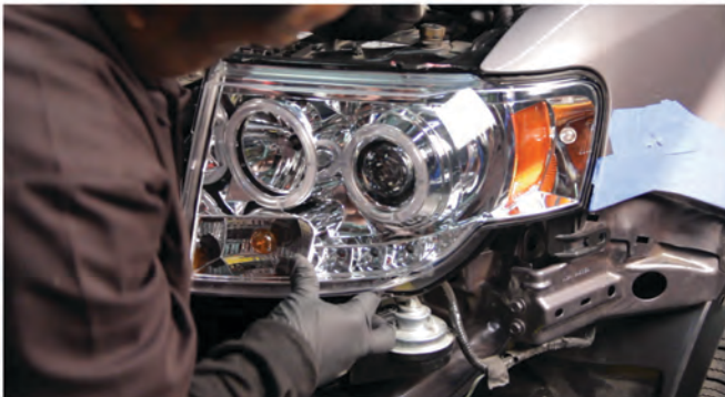
21) Seat the Spyder headlight being sure to snap the retainer tabs into place.
