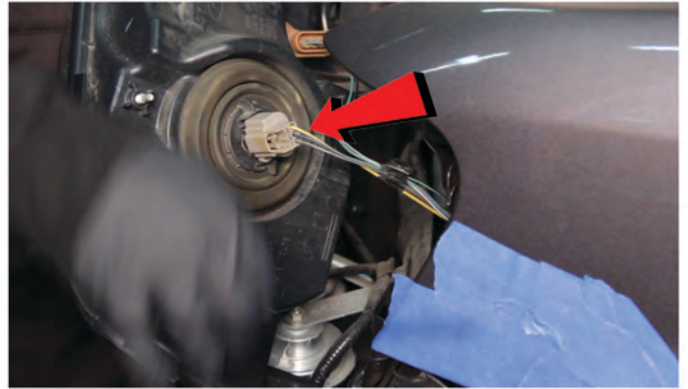
12) Disconnect the headlight harness.
