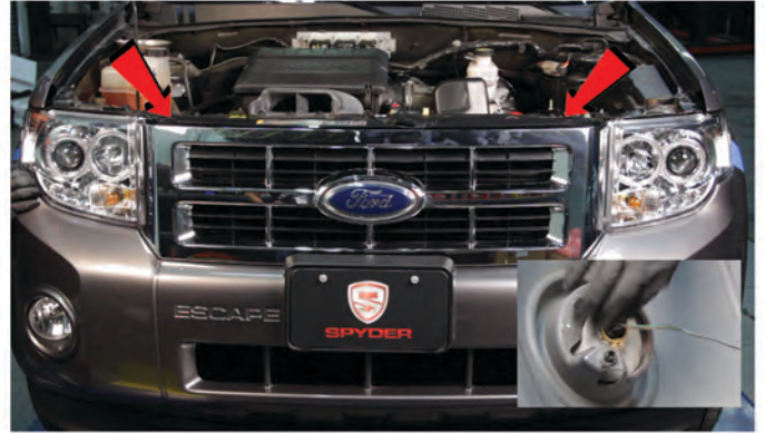
24) Seat the front bumper fascia and reinstall [2x] 10mm bolts above the grille to secure the fascia. Reconnect the fog light harnesses, if equipped.
