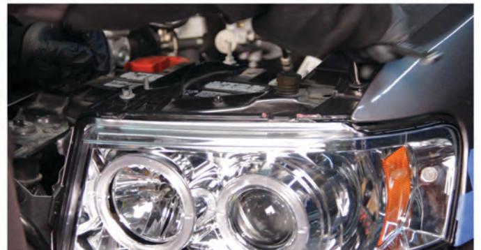
22) Reinstall [1x] 10mm nut & [1x] 10mm bolt securing the headlight from above.
