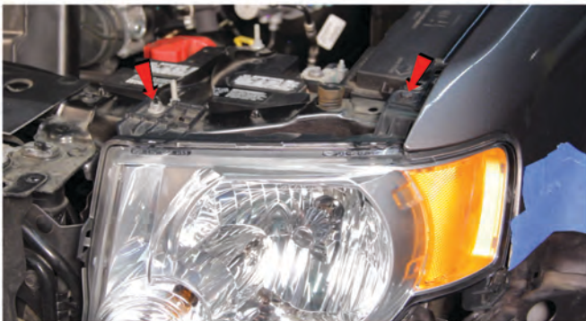
9) Remove [1x] 10mm bolt & [1x] 10mm nut securing the headlight from above.
