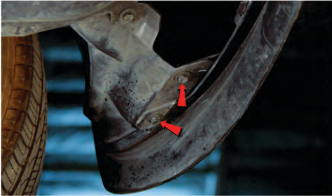
5) Remove [2x] 10mm bolts securing the fascia at the bottom corner on each side.
