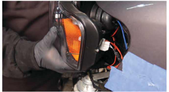
20) Reconnect the sidemarker socket.
