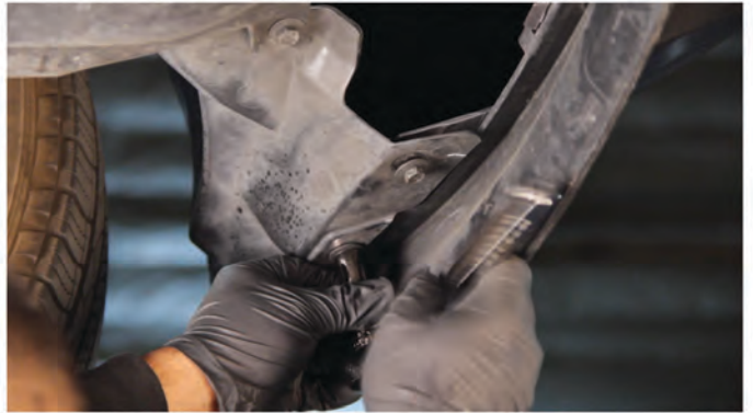
26) Reinstall [2x] 10mm bolts to secure the fascia at the bottom corner of the fascia on each side.
