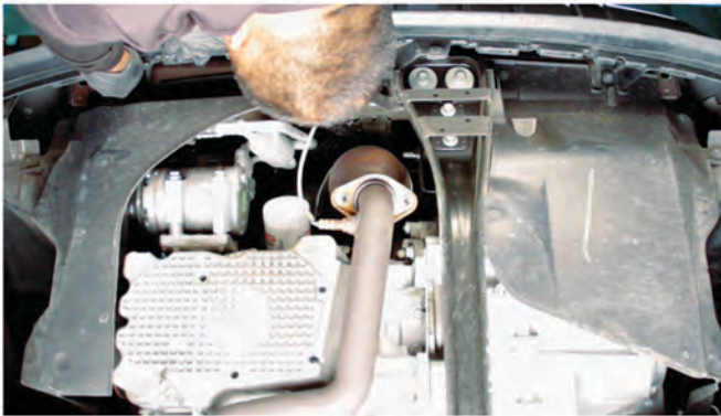
25) Reinstall [3x] 10mm bolts to secure the fascia to the undertray.
