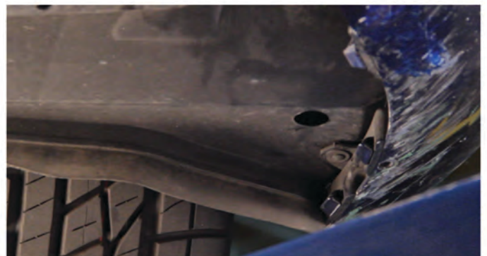
28) Reinstall [1x] plastic retainer to secure the bottom corner of the fascia to the undertray on each side.
