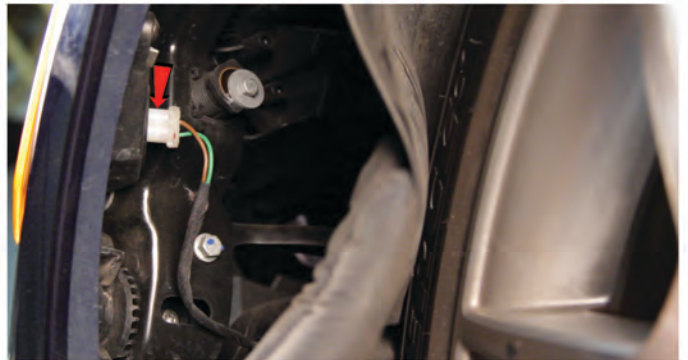
10) Disconnect the sidemarker harness.
