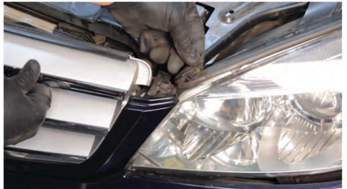
8) Release the headlight weatherstrip from the fascia by sliding it forwards to unhook it.
