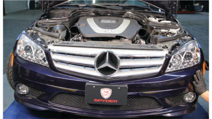
24) Seat the front bumper fascia being sure that its mounting tabs fit properly into place.
