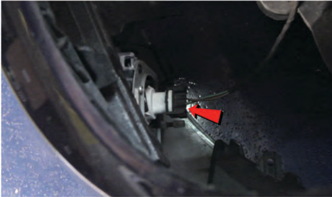
23) Reconnect the fog light wiring harness.
