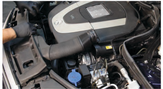
32) Seat the intake tube panel.
