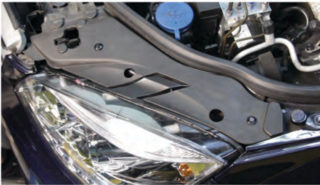
31) Replace the headlight filler panel and reinstall [2x] plastic retainers to secure the filler panel.
