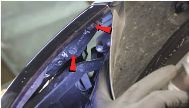
25) Reinstall [2x] 10mm bolts to secure the fascia to the fender.
