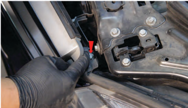
7) Peel back the weatherstrip and remove [1x] 10mm bolt next to the grille that secures the fascia.
