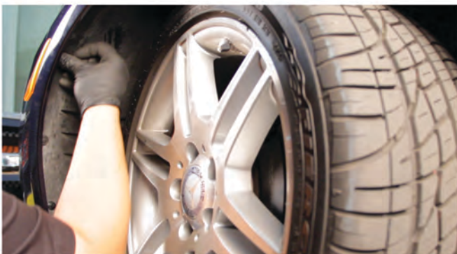
27) Reinstall [3x] plastic retainers in the wheel well to secure the fascia to the fender liner.
