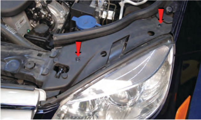
5) Remove [2x] plastic retainers that secure the headlight filler panel.
