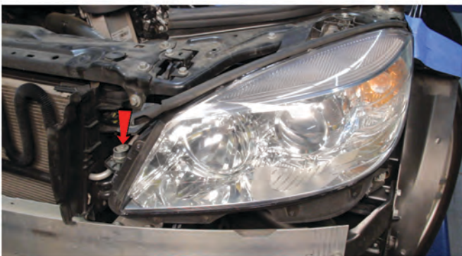
15) Remove [1x] 8mm bolt securing the headlight.
