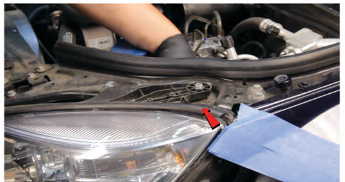
16) Remove [1x] 8mm bolt securing the headlight on the underside of the radiator core support.
