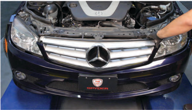
13) Peel back the edges carefully to unseat the front bumper fascia.
