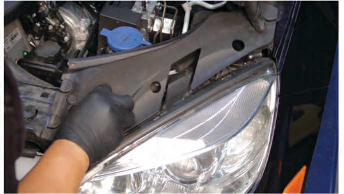
6) Remove the headlight filler panel.
