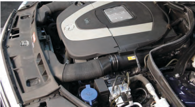
33) Reconnect the intake tubes and lock the retainer.
