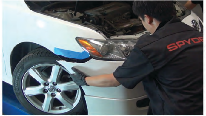
6) Pull upwards and away from the car to unseat the front bumper fascia.
