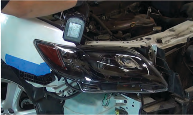
17) Reinstall [3x] 10mm bolts to secure the headlight.
