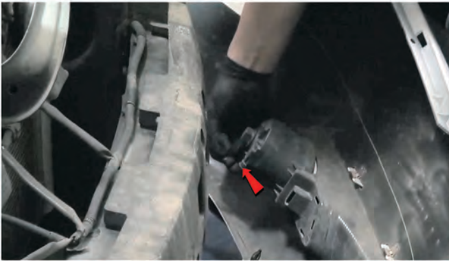
7) Disconnect the foglight wiring harness, then remove the fascia and set it aside.
