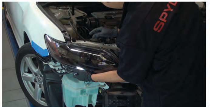
16) Seat the Spyder headlight, being sure to snap the mounting tabs fully into place.
