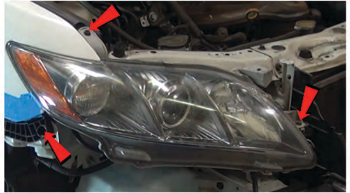
8) Remove [3x] 10mm bolts securing the headlight.
