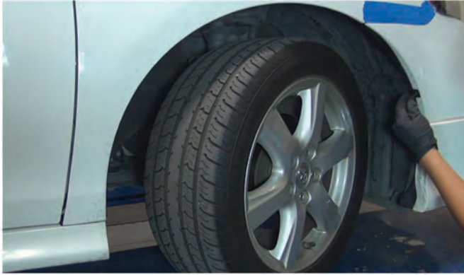
23) Seat the fender liner, then reinstall [1x] plastic retainer to secure the liner.
