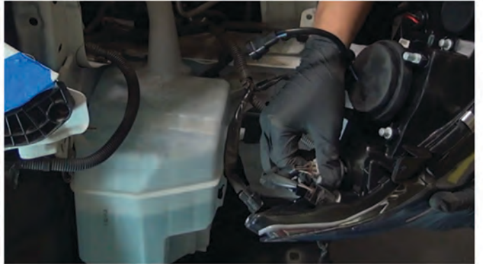
14) Reinstall the turn signal socket into the Spyder headlight.
