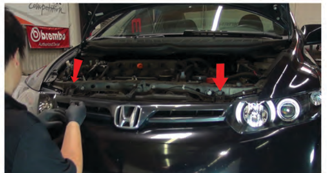
22) Reinstall two Size 5 Allen Key Screws Securing Upper Bumper Fascia.
