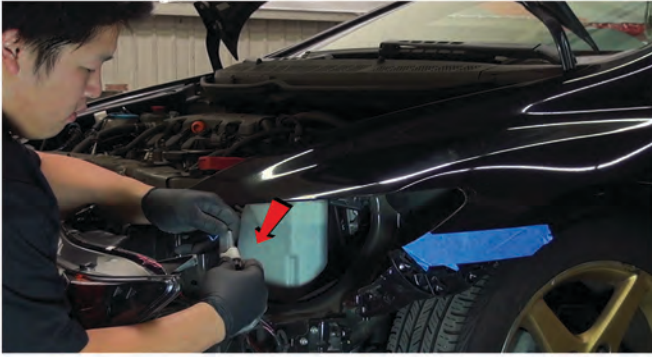
17) Reconnect High Beam & Low Beam Wiring Harnesses to SPYDER headlight and install turn signal bulb socket into SPYDER headlight.
