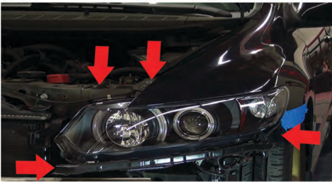
19) Reinstall four 10mm Bolts Securing Headlight
