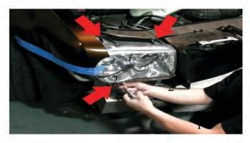
5) Now that the bumper has been removed locate the 3 10mm bolts that secure the head light down. There will be two on the top and one below. Use the 10mm socket or wrench to unscrew the from there bolt holes,
