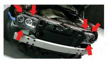
8) Tme to replace the head lights. Seat the head lights back into position by lining up the brackets to the mounting holes. Use the 10mm socket to fasten the 10mm bolts back. There should be 3 per side.
