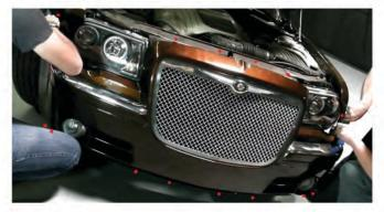
9) Place the bumper back by liining up the grill and corners with there mounting holes. You will need to replace the 4 clips on the grill, 10 mm bolt on both bumper corners, 4 clips on both sides of the fender liners and 8 8mm bolts on the bottom to secure the bumper back in place.
