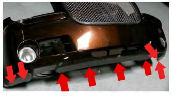
4) Before the bumper can be fully removed it will need to be detached from the slash guard. This is secured 4 8mm bolt on the outter edges of the bumper and 4 8mm bolts on the inner portion. You will need to use the 8mm socket or wrench to remove these from there bolt holes.
