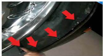
1) The bumper will need to be removeed to install your new Spyder head lights. First you will start by detaching the fender liner from the bumper. Use the Pannel Popper or Flat-head driver to pry the 4 clips from there mounting holes.
