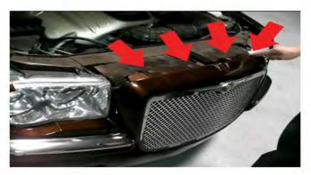
3) Now you will need to remove the top 4 clips fromg the grill area. Using the Pannel Popper or Flat-head driver again, pry the 4 clips from there mounting holes.
