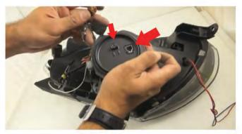
10) Next, take the HID harness and insert the clip into the ballast. Once properly connected, replace the harness back onto the ballast and screw the Phillips screw back down to secure the harness to the ballast.
