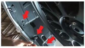
2) Once the fasteners on the grill have been removed, you will need to remove (3) plastic fasteners, shown here. remove and again set aside for later use.
