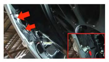
3) Next, you will need to remove (2) 10mm bolts that secure the bumper to the fender. Use the 10mm socket and ratchet to remove these. Also, you will need to remove the corner light bulb and socket from the bumper shown. Simply twist counter clockwise to unlock. Repeat this process for both sides.
