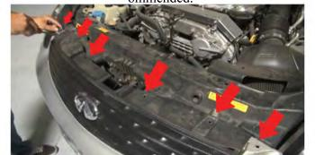
1) Begin by opening your hood and locate the (6) plastic fasteners. Using the panel popper tool, gently pry the bolts free and set them aside for later.
