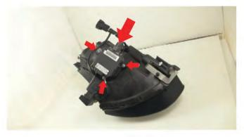
6) You will need to use some components from your original head lights to transfer to your new Spyder head lights. Start by unscrewing (3) Phillips screws from the ballast shown, then unsnap the harness clip from the ballast and flip over.
