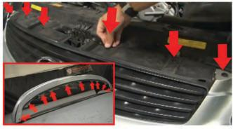
15) Next, replace the 6 Plastic fasteners on the grill area to secure it down. Lastly, replace all (10) 10mm bolts to secure the splash guard and bumper back to the frame.
