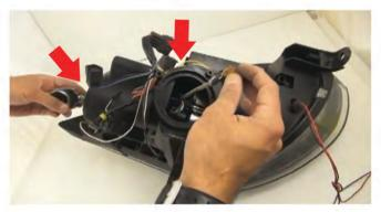
9) The next step is to thread the HID bulb harness through the head light from the low beam socket to the opening where the ballast will sit.
