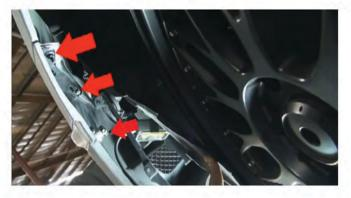
14) Now we will be reinstalling the bumper with plastic fasteners and bolts. Start by replacing the (2) 10mm bolt that secure the bumper to the fender. Then replace the corner light socket in the corner light housing.
