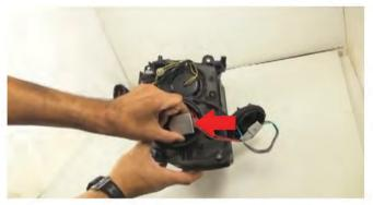
8) Now on the back of the head light, remove the low beam backing to expose the HID bulb and harness socket. Remove the socket by gently wiggling if from the bulb. Once released from the bulb, pull the HID bulb harness all the way out and set net to your ballast. unclip the bulb and remove. \*\*\*DO NOT TOUCH THE BULB\*\*\*. Set aside with the ballast and HID harness.
