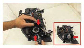
12) Next, you will need to remove the clip from your OEM head light and clip it to your new Spyder head lights, Replace the HID bulb not touching the glass of the bulb. secure the bulb with the clips. Next plug the HID harness socket to the back of the bulb as shown.
