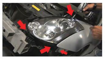
5) In order to remove the head light you will need to unbolt (4) 10mm bolts holding the head light in place. Once removed, unplug the head light wiring harnesses to completely remove the head light.
