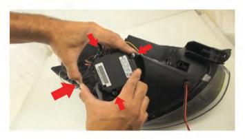
11) Replace the ballast by lining up the mount holes with the screw hole on the back of the head light. Screw the (3) Phillips screws to mount the ballast, connect the power socket to the ballast from the head light
