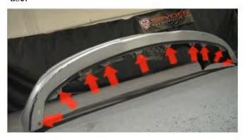
4) Before the bumper can be fully removed you will need to remove a total of (10) 10mm bolts from the bottom of the bumper to release it from the splash guard. Once they have all been removed gently pull the bumper from the frame and set it where it cannot get damaged.
