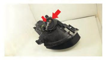
7) The next step is to unscrew (1) Phillips screw from the ballast to release the HID bulb harness. After you have done this pull out the HID bulb harness from the ballast. Keep the ballast close you will be needing this for your Spyder lights.
