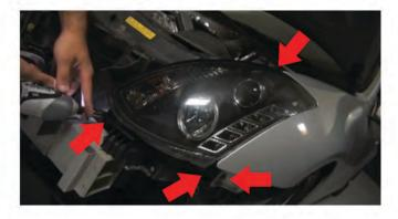
13) The next step is to connect the OEM harnesses to the new Head lights. After that, seat the new head light on to the vehicle lining up the mount holes with the bolt holes. Replace the (4) 10mm bolts to secure the head light to the vehicle.
