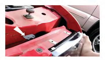
10) Seat the SPYDER headlight, then push down on the inner retainer tab to lock the headlight into place.
