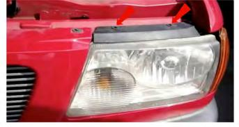
1) Remove two 5.5mm Bolts Securing Headlight Trim Cover.
