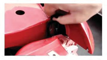
8) Remove the outer retainer tab and discard it.
