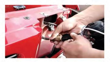
9) Connect the SPYDER headlight harness to the factory wiring harness.
