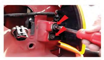
6) Remove two 5.5mm Screws securing the corner lamp.
