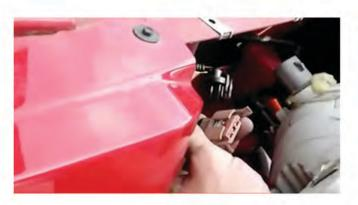
5) Disconnect the headlight and park light/turn signal harnesses from the headlight sockets.
