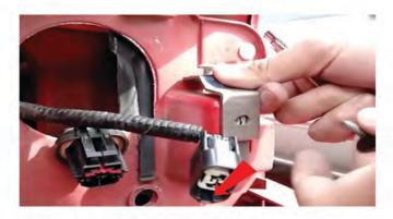
7) Locate the special bracket included with your SPYDER headlight. Install the bracket as shown in the location where the corner lamp bracket used to mount.
