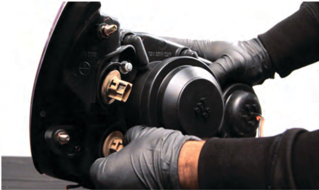
35) Reinstall [2x] turn signal sockets into the Spyder headlight.
