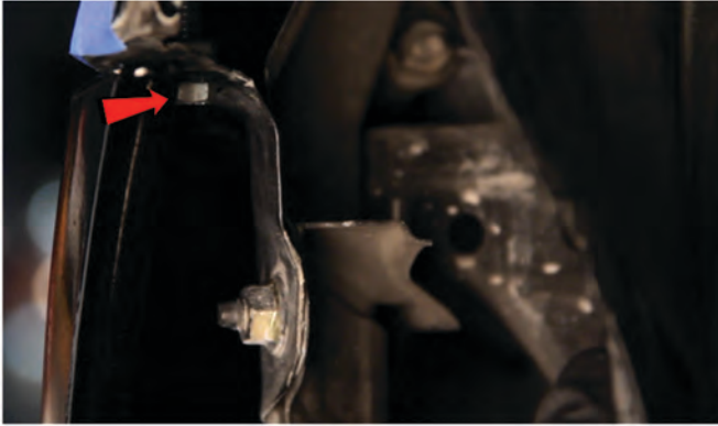
5) Remove [1x] 10mm bolt that secures the fascia to the fender.
