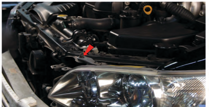
10) Remove [1x] 10mm bolt securing the headlight.
