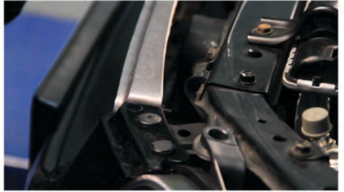
48) Reinstall [2x] phillips and [2x] pry-out plastic retainers on either side of the grille to secure the fascia.
