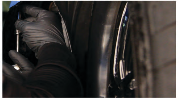
50) Reinstall [1x] 10mm bolt to secure the fascia to the fender in the wheel well.
