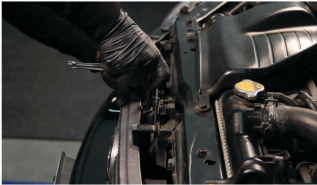
49) Reinstall [1x] 10mm bolt next to the hood latch to secure the fascia.
