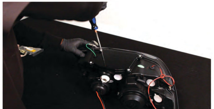
28) Remove the [4x] phillips screws securing the ballast cover from the Spyder headlight, then remove the Spyder ballast cover and discard the Spyder ballast cover, as the OEM ballast cover will be used.
