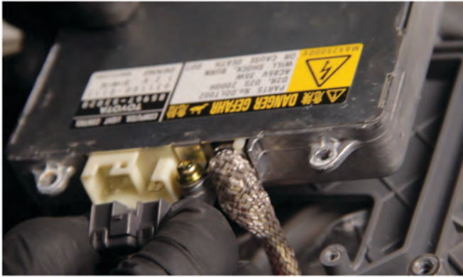
23) Disconnect the HID input harness from the ballast.
