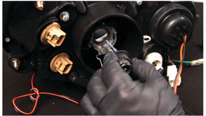
36) Install the HID bulb into the Spyder headlight, then lock the bulb retainer.
