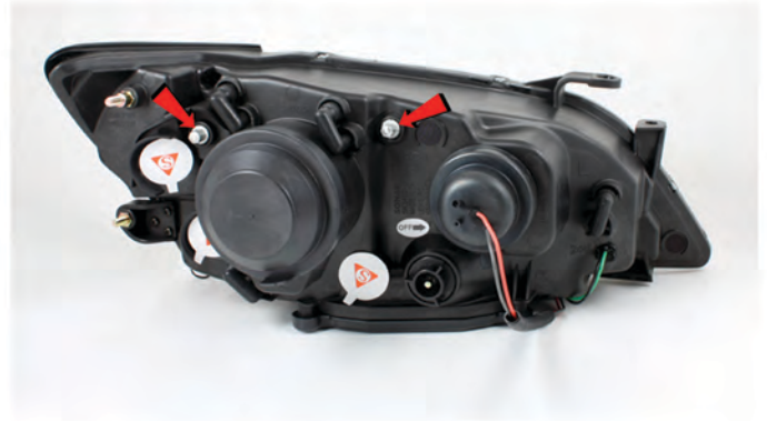
38) Your beam adjusters are marked here and are 8mm. For information on how to wire the halos and more, watch How To Wire Halos in the Spyder FAQs Playlist on the Spyder Auto YouTube channel.
