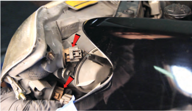
13) Disconnect the turn signal harnesses.
