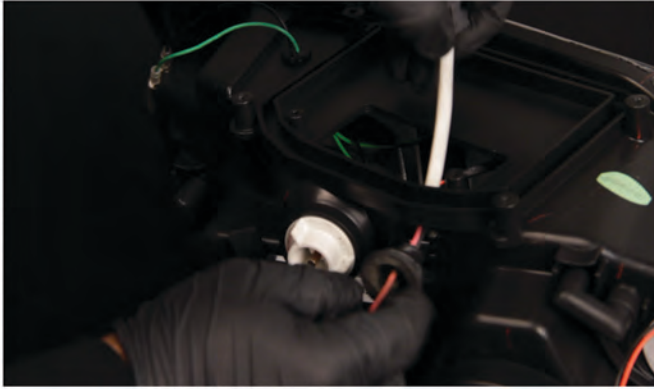
29) Feed the HID input harness into the Spyder headlight, being sure to seat the grommet fully into the headlight to prevent condensation issues.
