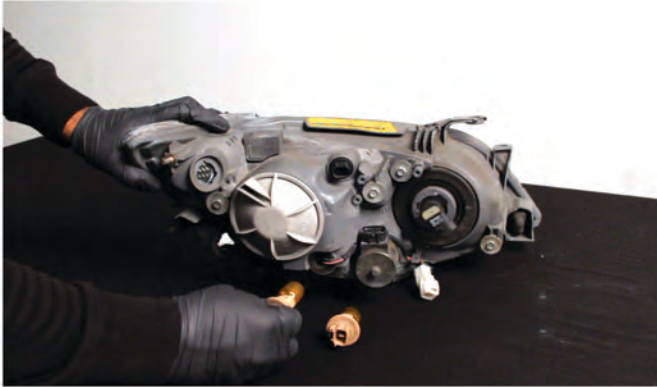
17) Remove [2x] turn signal sockets from the OEM headlight. Never touch exposed bulbs with bare hands.
