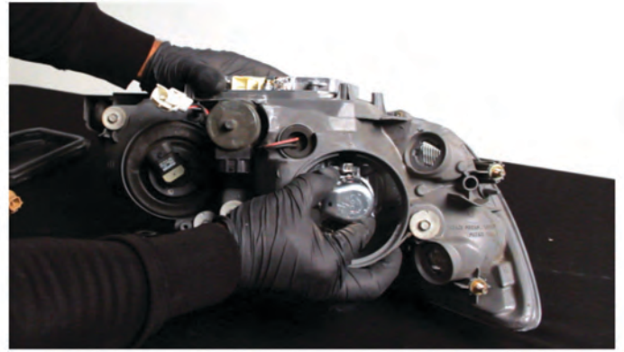
24) Disconnect the Ignitor wire (ballast harness) from the HID bulb.
