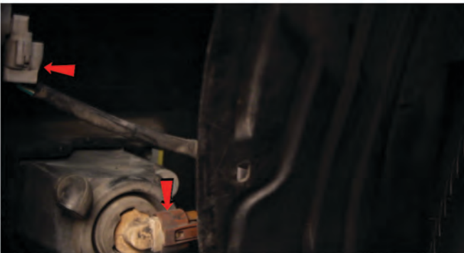
9) Disconnect the sidemarker and fog light harnesses.
