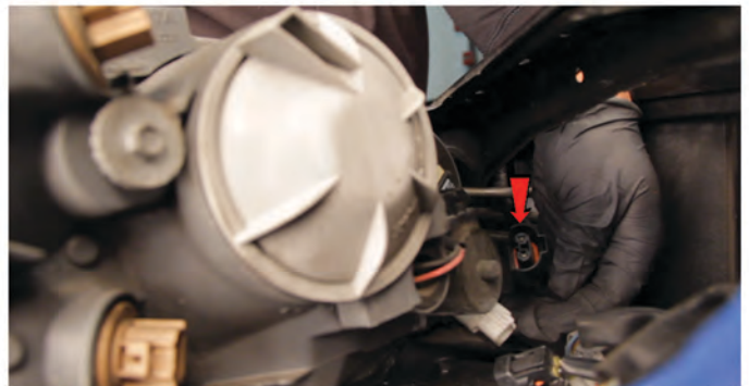
16) Disconnect the high beam harness.
