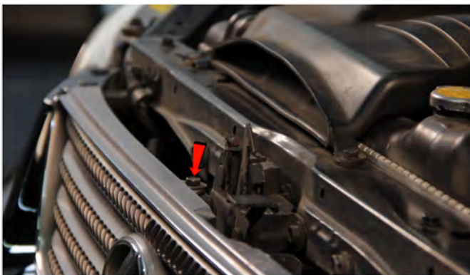
3) Remove [1x] 10mm bolt next to the hood latch.
