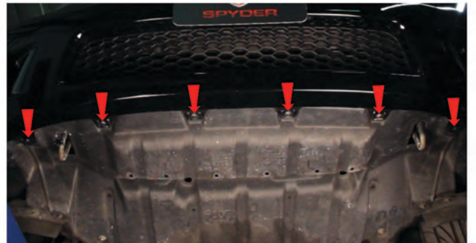
52) Reinstall [6x] 10mm bolts to secure the fascia to the undertray.
