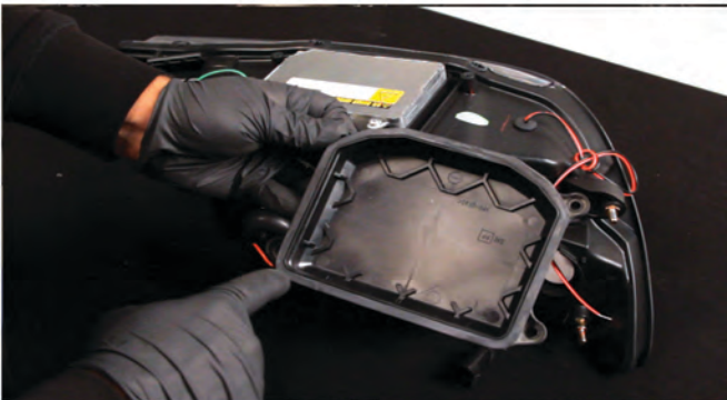
33) Locate the OEM ballast cover. Inspect the gasket, replace the gasket if it's damaged or worn.
