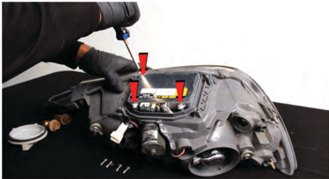
21) Remove [3x] phillips screws securing the ballast to the headlight.
