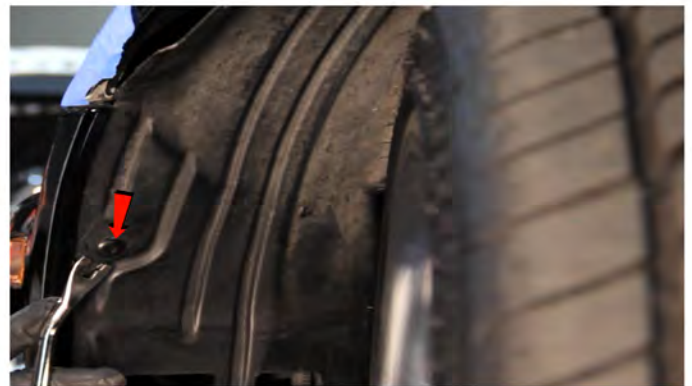
4) Remove [1x] plastic retainer securing the fender liner.
