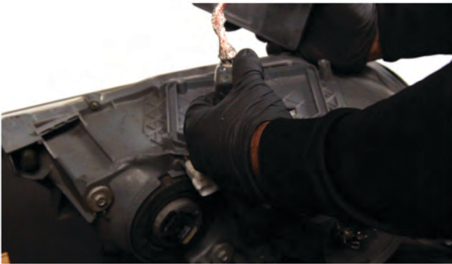
25) Remove the ballast and Ignitor Wire from the OEM headlight.
