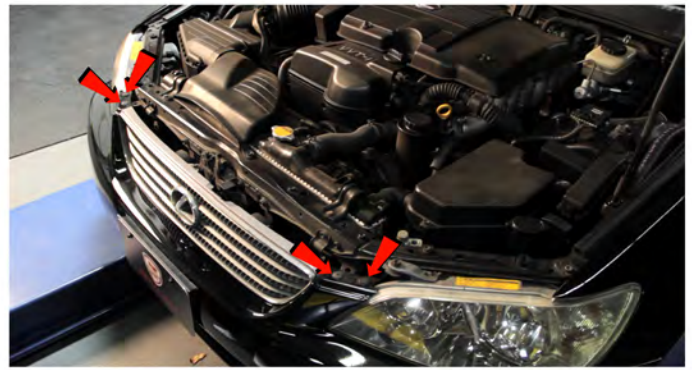
2) Remove [2x] phillips and [2x] pry-out type plastic retainers securing the fascia.
