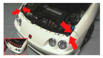
2) Next, you will have to remove the (4) 10mm bolts one on top and another on the side. Next remove the (9) screws on the grill area that hold down the mount plat and bumper.
