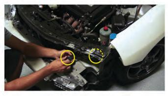
5) After the head lights have been removed, gently remove the inner hi-beam bulb from its sockets shown by the solid circle. Leave the low-beam bulbs in their sockets shown by the dotted circle.
