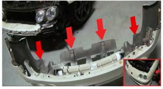
3)Before the bumper can be fully removed you will need to take off the (4) 10mm bolts that hold the splash plate and bumper to the bottom of the frame. Once these have been removed there will be (1) 10mm bolt on both sides of the bumper that hold it to the fender. Now, you can remove the bumper.
