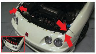
8) Next, seat the bumper, lining up the mount holes with their bolt holes. Replace the (4) 10mm bolts, one on top and another on the side to both sides. Next replace the (9) screws on the grill area to bolt down the mount plat and bumper.
