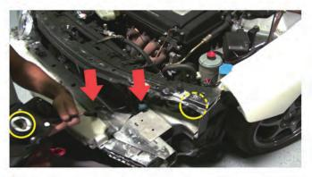
6) Take your new Spyder lights and plug in the Hi-beam harness into the hi-beam socket of the lights. Next take the low-beam bulbs and simply seat them in the heal light and twist them counterclockwise to secure them tight. doing this properly prevents condensation in the head lights.
