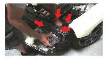
7) Now it is time to seat the new lights. Seat them by lining up the mount holes to the bolts holes on the vehicle. Using your existing (4) 10mm bolts bolt the head light down.
