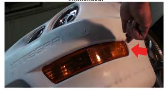
1) First you will need to start by removing the corner bumper lights. Use the screw driver to unscrew the screw from its mount hole. Remove the bumper light and twist of the sockets lights. Set the light aside.
