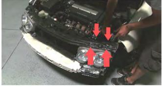
4) Now to remove the head lights. there will be (2) 10mm bolts behind the head light and (9) 10mm bolts on the top. Remove these and set them aside with the others. Untwist the Hi and Low beam bulbs from your OE head lights, set the head light aside.
