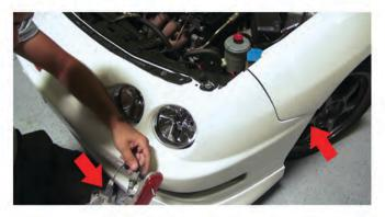
9) Finally replace the (4) 10mm bolts on the bottom of the bumper and the (1) 10mm bolt to secure the bumper to the fender on both sides. Replace the corner bumper lights placing the bumper light harnesses and bulbs into their sockets, twist the sockets lights tightly. Use the screw driver to screw the screws back in the
