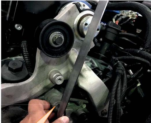
Align steel rule to the mounting face
