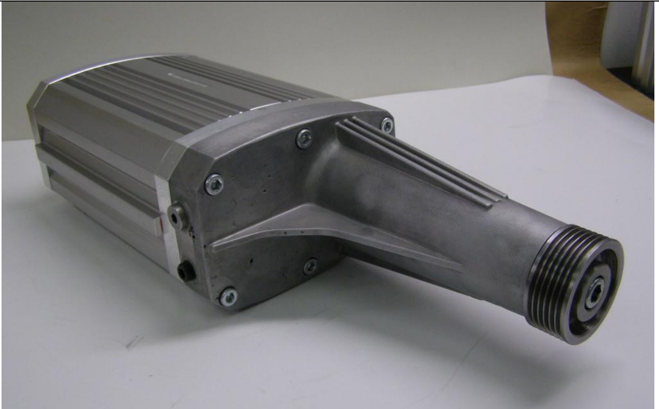
Front view showing the long extension housing with pulley
