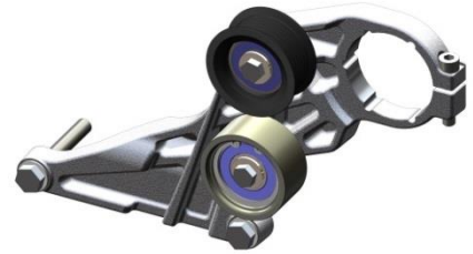
Supercharger drive support bracket with ancillary hardware
