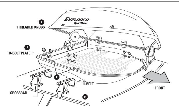
When carrier is assembled, place on the crossrails, place U-Bolts (H) under crossrails and assemble U-bolts through Carrier bottom mounting holes and U-bolt plates (J). Secure with threaded knobs (I). Recheck to see that your crossrails are securely locked into position. For safety the hooks in the carrier locks must properly engage the lock brackets (E) whenever the vehicle is in motion.
