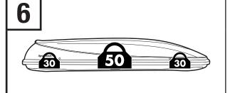
Make sure that loads are evenly distributed inside the roof box. Do not exceed the maximum
