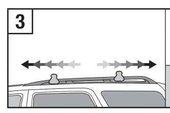
If crossbars are adjustable, set to widest position which can be accommodated by mounting slots.
