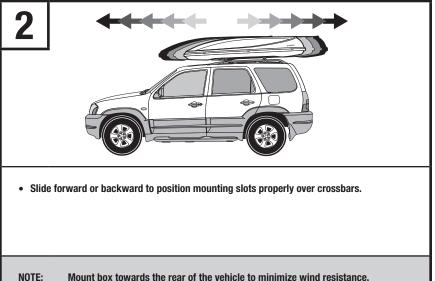
Mount box towards the rear of the vehicle to minimize wind resistance.
