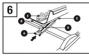
• When you are ready to mount the carrier to the vehicle's roof rack crossrails,slide each saddle until it separates from the carriage bolt and drops down.
