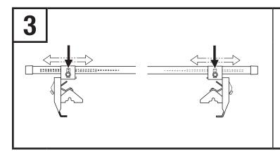
• Using the included fit chart, adjust foot positions to the numbers for your vehicle. Use "Front" dimensions for front bar and "Rear" for rear bar.
