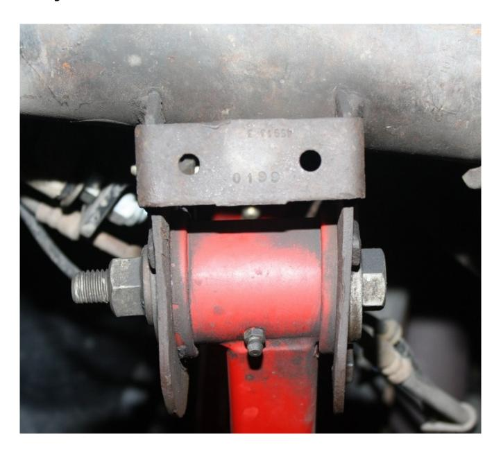
Spohn Performance front lower control arm skid plate installed
