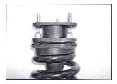
11. Locate (3) 3/8" flanged head lock nuts from the hardware bag. Working on the driver's side, install the newly modified stock strut into the stock upper location. **Do not tighten at this point**. Secure the lower portion of the strut to the stock lower control arm using the stock hardware. **Do not tighten at this point**.
