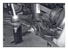
10. Locate (1) new strut spacer and the stock hardware that connected the stock strut into the stock location. Install the new spacer on top of the stock strut and secure using the stock hardware. Make sure to use Loctite and torque to 45 ft/lbs.
