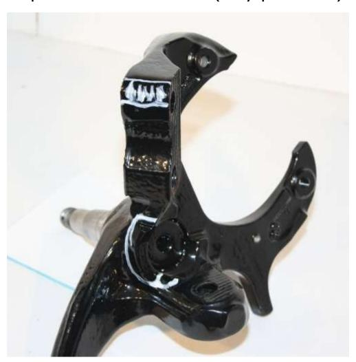
Step 2: After Grinding The Spindle (Heavy Spindles Shown)
