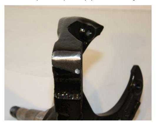
Finished: We Have Now Gained The Clearance Needed To Mount The Strut
