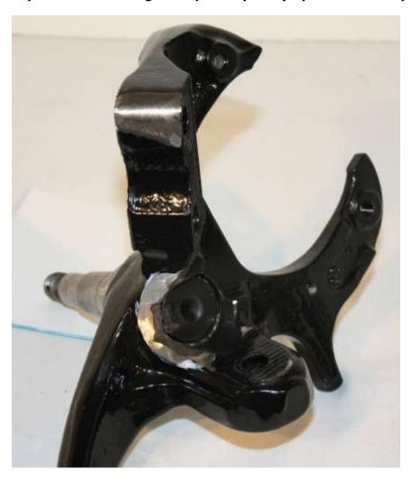
**Clearance Required For Bottom Adjuster Housing (All Spindles)**
