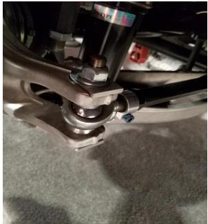
3. Install the provided Eccentric Lockout Washers (7) in the subframe. They should fit between the two grooves in the subframe and prevent the bolt from moving.
