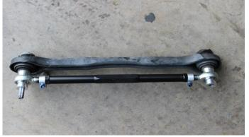
2. Set SPL Parts Rear Toe Arm next to the OEM arm. Use the bolts through the stock arm to set the SPL Parts Arm to the exact length of the OEM arm ensuring equal thread engagement on both ends. **Note:** the groove on one side of the arm to indicate the left-hand threaded side.
