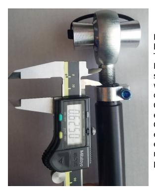
Loosen the Aluminum Clamps (6) on both ends of the Turnbuckle. Turn the Turnbuckle so as to thread in/out the FK Rod End (spherical bearing side). Threading in/out the FK Rod End will in turn thread out/in the Turnbuckle on the chassis side. Once the FK Rod End is long/short enough, tighten down the Aluminum Clamps. Note that for safe thread engagement, the **maximum** amount of exposed thread on the Rod End should not exceed the measurement as pictured on the left.
