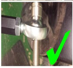
Note that the FK Rod End can rotate freely, so the picture on left is not binding even though the edge of the ball is touching the housing.
