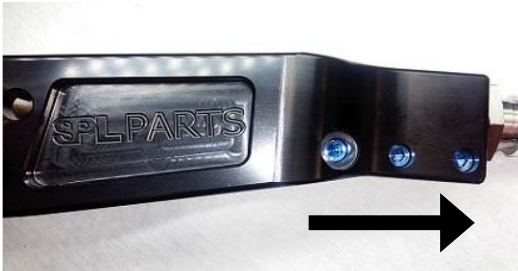
Tighten Blue Anodized Titanium Head Cap Screws starting from the "SPL Parts" logo, working towards the FK Rod End
