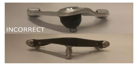
The images above show the correct way to determine what arm goes on what side of the vehicle. Match up the SPL arm with the OEM arm by observing the canted ball joint. This will allow proper articulation of the ball joint.
