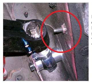
Here is a picture of the bolt that holds down the power steering reservoir. Make sure to replace this bolt with a shorter one or grind this bolt down as you may encounter contact issues when reducing caster.
