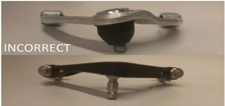
The images above show the correct way to determine what arm goes on what side of the vehicle. Match up the SPL Parts arm with the OEM arm by observing the canted ball joint. This will allow proper articulation of the ball joint.
