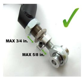
The next picture shows a properly threaded adjuster. The rod end (heim joint) will thread out about 2/3 the length of the adjuster. The maximum adjustment limits are shown in the picture. This jam nut should be tightened against
