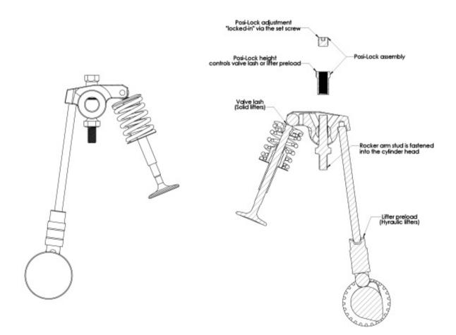
If the engine is complete and installed in the vehicle, run the engine until normal operating temperature is reached. This is referred to as "hot" adjustment. "Cold" adjustments should only be
