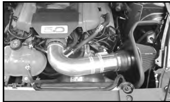
Step 19 Reinstall the engine cover. Make sure that all clamps and hardware are fully tightened. Reconnect the battery cable, start the vehicle and let it warm up. Shut off and inspect the installation once more for any loose clamps, wires, or hardware. Test drive & enjoy! Your installation is now complete. Periodically check all clamps and brackets.
