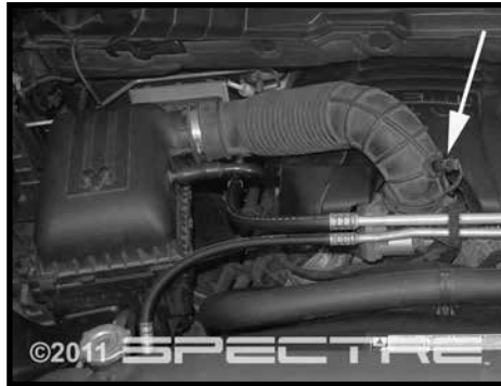
Step 2 Disconnect the IAT sensor connector.
