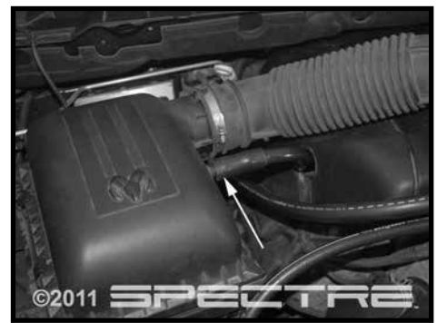
Step 3 Disconnect the PCV breather hose from the airbox lid.
