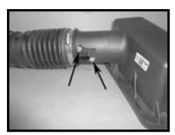
Step 5 Remove the MAFS from the factory intake tube
