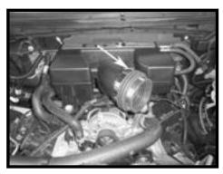
Step 9 Install the flex coupler on the plenum and secure the coupler in place. Install a second clamp but do not tighten at this time.
