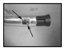
Step 6 Install the MAFS into the Spectre Performance aluminum intake tube, then install the MAFS Sleeve(Patent No. 7,681,461) into the aluminum intake tube.
