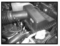
Step 4 Unclip the three hold down clips on the air filter lid, lift the lid then slide it forward to clear the locking tabs. Remove the air filter lid/intake tube assembly and air filter.
