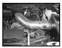
Step 10 Install the Spectre Performance intake tube into the coupler on the heat shield then into the flex coupler on the throttle body. Fasten securely in place
