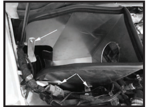
Step 10 Install the heat shield using the supplied hardware and fasten securely once in place.
