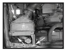
Step 6 Loosen the three bolts securing the air box assembly to the vehicle. Remove the factory intake from the vehicle.
