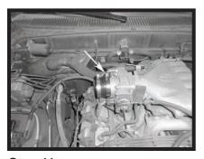
Step 11 Install the coupler on the throttle body. Tighten the clamp on the throttle side and make sure the intake side clamp is installed but left loose.
