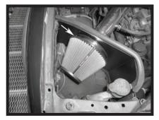
Step 16 Install the filter and fully tighten the clamp.
