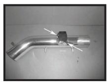
Step 8 Insert and fasten the MAFS onto the Spectre Performance intake tube with the provided machine screws.
