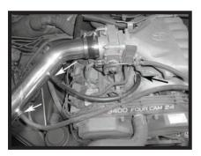
Step 15 Reconnect the existing hose to the intake tube. Using the supplied 1/4" hose, connect the hose to engine and to the intake tube as shown.
