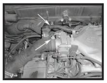
Step 3 Remove the 1/2" breather hose from the back of the factory intake. Loosen the clamp at the throttle body.
