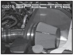
Step 23 Install Spectre air filter and fasten securely with supplied hose clamp. Ensure that all clamps and hardware are fully tightened at this time.
