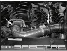
Step 18 Install the long intake tube into the throttle body coupler and then slide the 3.5" coupler back over from the short tube. Once tubes and couplers are in position, securely fasten all clamps.
