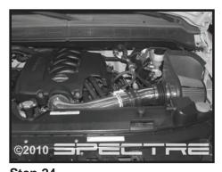
Step 24 Make sure that all clamps and hardware are fully tightened. Reconnect the battery cable, start the vehicle and let it warm up. Shut off and inspect the installation once more for any loose clamps, wires, or hardware. Test drive & enjoy! Your installation is now complete. Periodically check all clamps and brackets.
