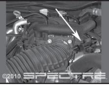
Step 2 Disconnect the air temperature sensor by releasing the locking tab and disconnect.
