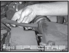
Step 3 Disconnect the crank case vent hose from the stock intake.
