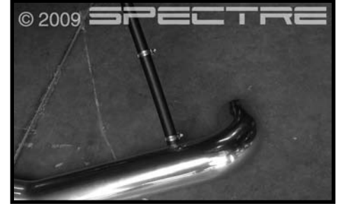
Step 11 Install the supplied breather hose onto the Spectre intake and secure with the supplied clamp. Install the second clamp onto the hose, but leave loose at this time.
