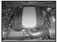
Step 2 Remove the engine cover.
