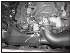
Step 5 Disconnect the electrical connector on the intake air temperature sensor. Loosen the clamp at the throttle. Remove the factory air intake system from the from the sensor. vehicle.
