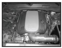
Step 15 Install top engine cover. Position the breather hose so it does not rub on cover.
