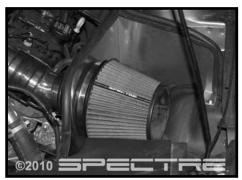
Step 19 Install the air filter and clamp to the velocity stack adaptor. Verify all hardware and clamps are fully tightened.
