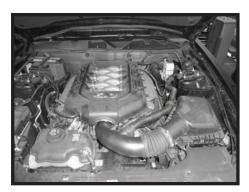
Step 2 Remove the engine cover by lifting on all the corners.
