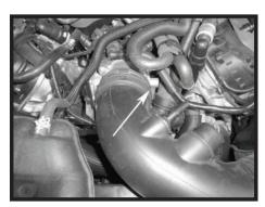
Step 5 Loosen the hose clamp at the throttle body.
