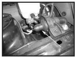
Step 19 Install the supplied cap over the valve that the roar tube was removed from in Step 4.
