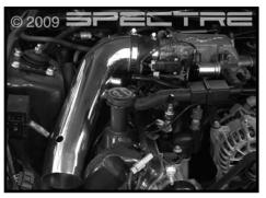
Step 9 Install the Spectre intake tube as shown. Do not fully tighten clamp at this time.
