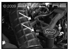
Step 3 (continued) Disconnect the two hoses from the stock intake (as shown) and remove the stock intake.
