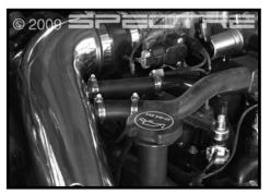
Step 10 Install the two hose pieces to the If your vehicle has an Intake Air intake and stock tubes. Secure with the included clamps.
