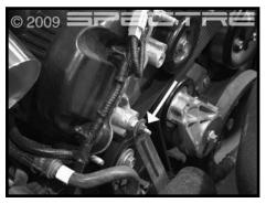
Step 14 Loosen, but do not remove the nut shown below.
