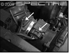
Step 2 Unplug the wires from the mass air flow sensor (MAFS) and intake air temperature (IAT) sensor.
