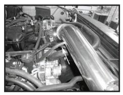
Step 18 Install the new hose onto the vacuum fitting on the intake tube.
