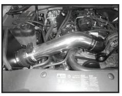
Step 16 <u>Install the intake tube</u> as shown and once in position tighten clamps.
