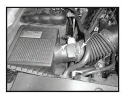
Step 4 Loosen the clamp at the Mass Air Flow Sensor (MAFS). Disconnect the MAFS electrical connector.
