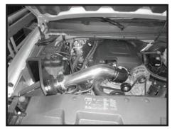
Step 20 Reinstall the engine cover. Make sure that all clamps and hardware are fully tightened. Reconnect the battery cable, start the vehicle and let it warm up. Shut off and inspect the installation once more for any loose clamps, wires, or hardware. Test drive & enjoy! Your installation is now complete. Periodically check all clamps and brackets.
