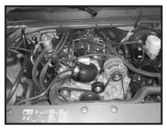
Step 13 Install the 90° boot on throttle body with the short side on the throttle body and clamp on the throttle body side to secure the boot in place. Install a second clamp but do not tighten at this time.
