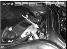
Step 11 Install the vent hose on the intake tube.
