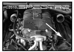
Step 8 Install the supplied vent hose as shown on the valve cover nipple.
